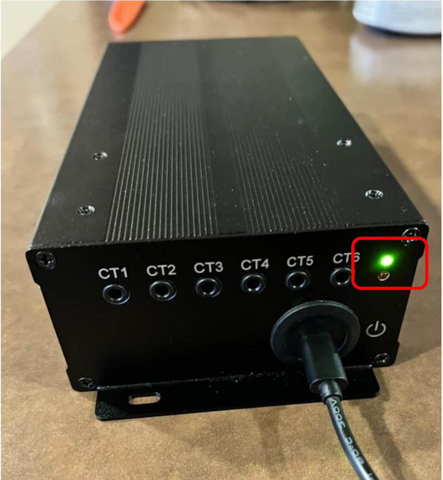
10. Confirm the LED on the EMS controller is solid green – meaning the EMS is connected to the back end.
